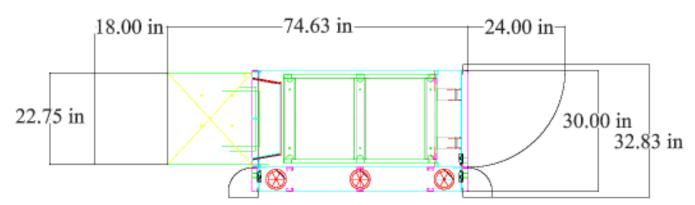
iii. R.A.S.E.R. DX footprint and minimum clearances (without Mission Critical Venting Installed).
