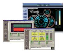
**Communication software** allows not only the control of the UPS and its smooth shutdown when Utility fails, but also allows the user to
