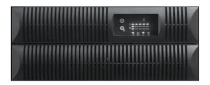
Both the XPRT-6kVA model (4U) and the XPRT-10kVA (6U) are the smallest available solutions including hot-swappable internal batteries, automatic bypass, integrated maintenance bypass, and dual-voltage output. XPRT dual-inverter design provides simultaneous output voltages of 240/120V, 208/120V, 230/115V, 220/110V, or 200/100V without the need for transformers saving space, weight, and power.
