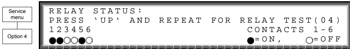
Figure 90: Service – setting alarm contacts
