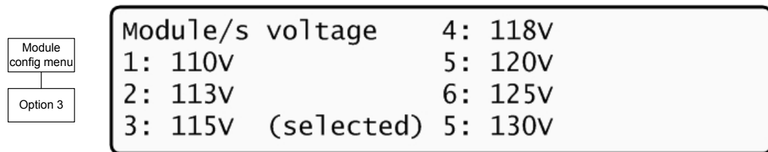
Figure 61: Setting the module voltage
