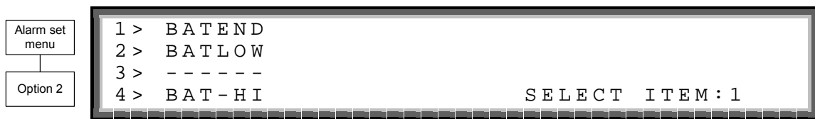
Figure 52: Battery parameters for alarm
